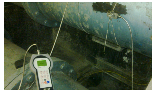
KATflow 200 installed on large sewage pipe
